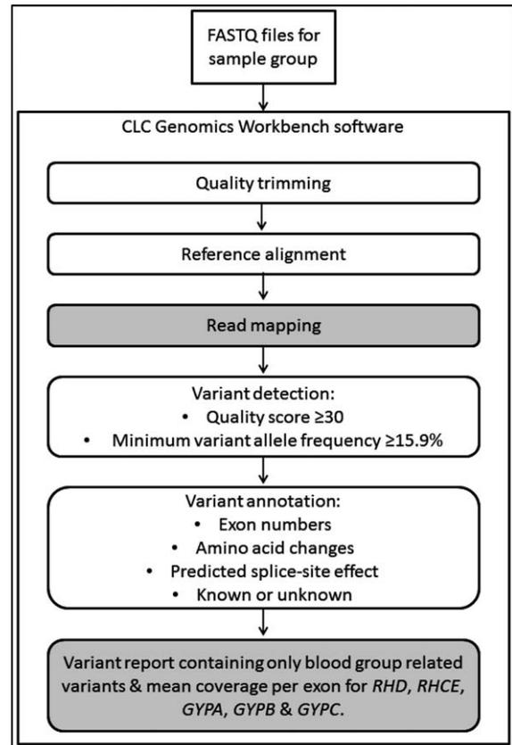
**Fig. 1. Overview of secondary data analysis using the CLC Genomic Workbench software. White rounded rectangles = processes; gray rounded rectangles = data output files.**
